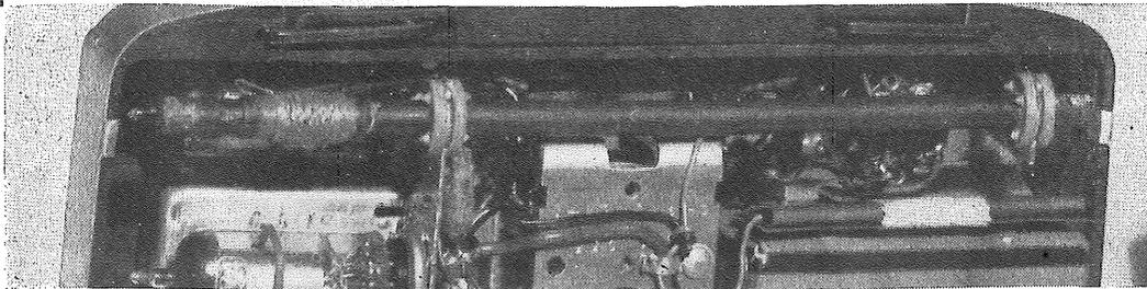
An RCA personal portable receiver showing relative size and location of antenna near top
